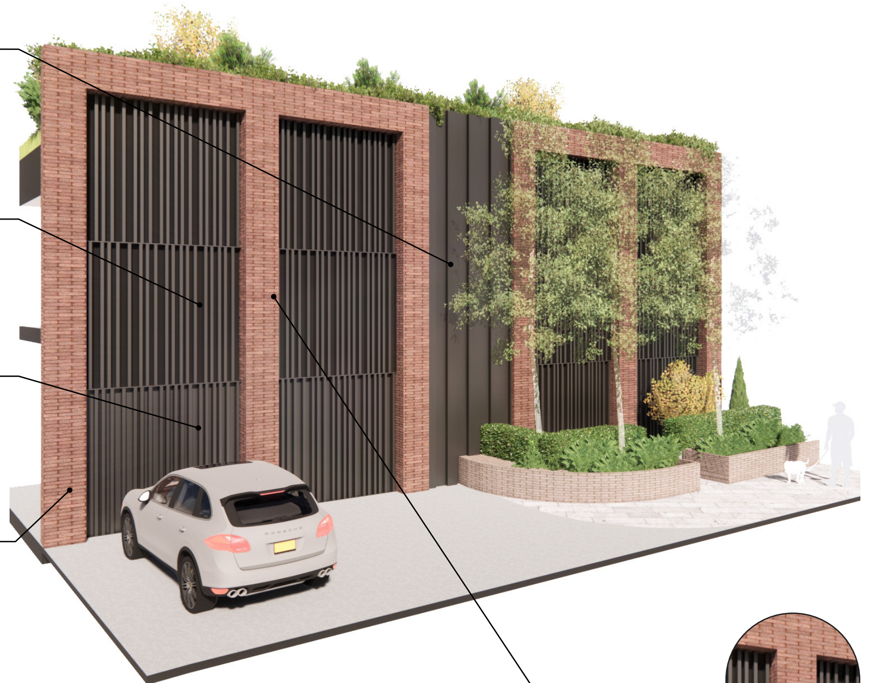
Additional brick pier added to enhance facade rhythm and emphasise vertical expression
